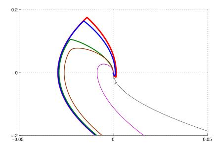
Figure 2: Optimal solutions of the perturbed Fuller's problem associated with different values of  $\varepsilon$  ranging from  $10^{-7}$  to  $10^{-2}$  as in Table 1. Thicker lines corresponds to smaller values of  $\varepsilon$ . The optimal Fuller's trajectory  $x_0$  is represented by the dashed line.
